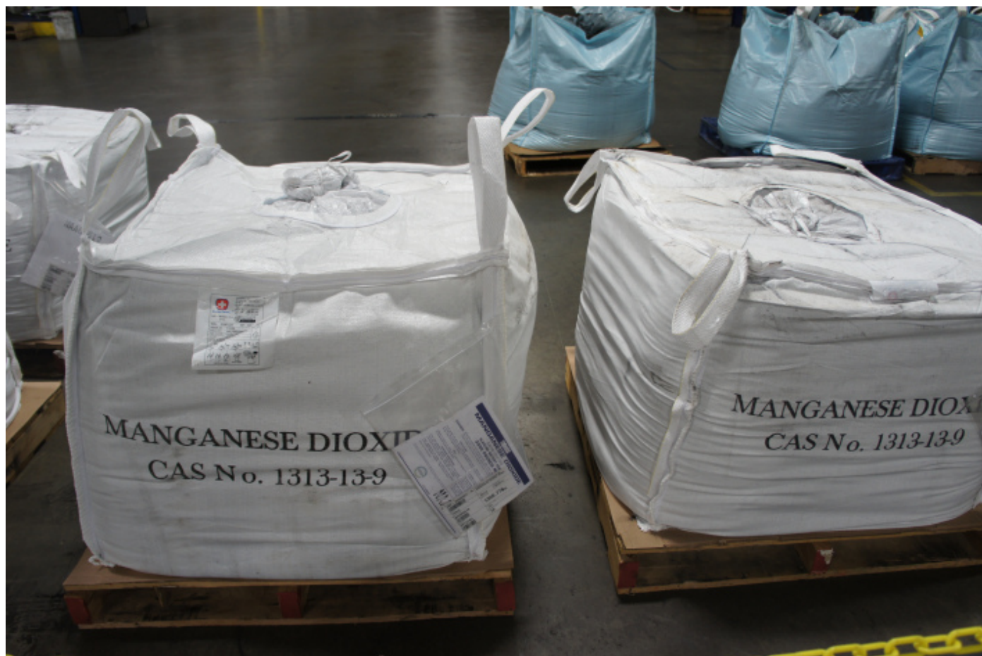
Material powders that go into Aquion's electrodes. Image courtesy of Katie Fehrenbacher, Gigaom
