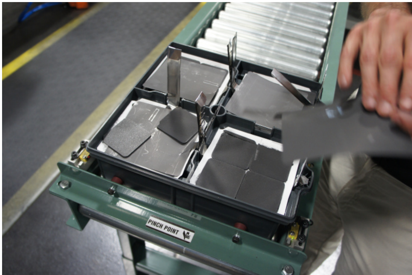
Inside of an Aquion Energy battery, showing the cathode and anode pairs. Image courtesy of Katie Fehrenbacher, Gigaom.
